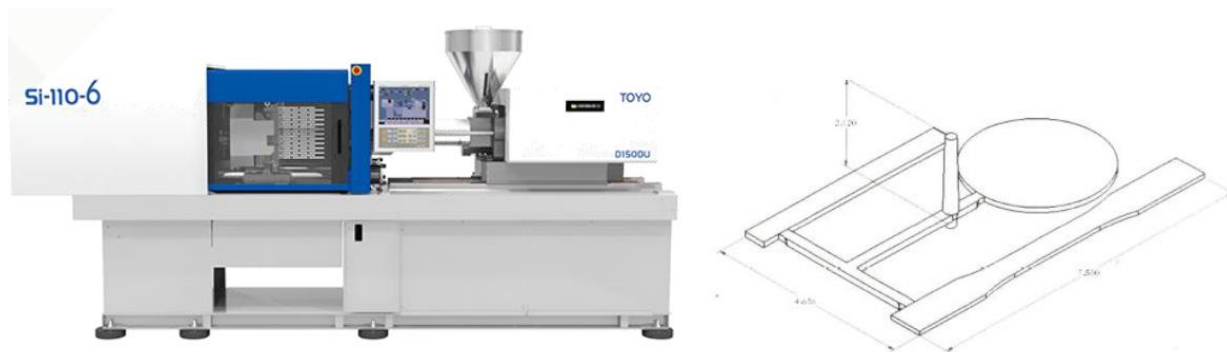
Figure 8: Injection molding machine and molded ASTM standard specimens
