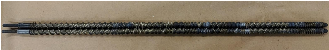
Figure 7: Screw configuration in extrusion compounding
