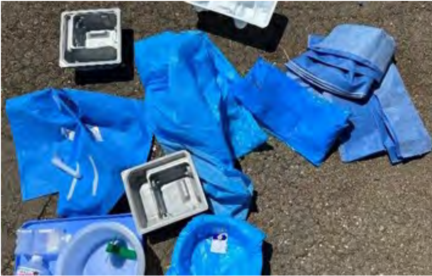
Figure X: Remaining PE, PP, and PS parts after sortation that were used for feedstock testing by Resynergi.
