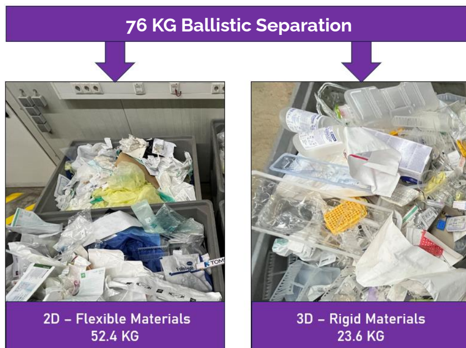
Figure 4. Results of ballistic separation
