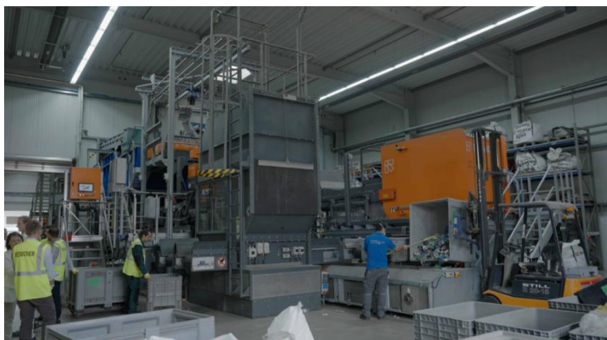
Figure 1. Ballistic separation unit to segregate flat, flexible from rigid materials
