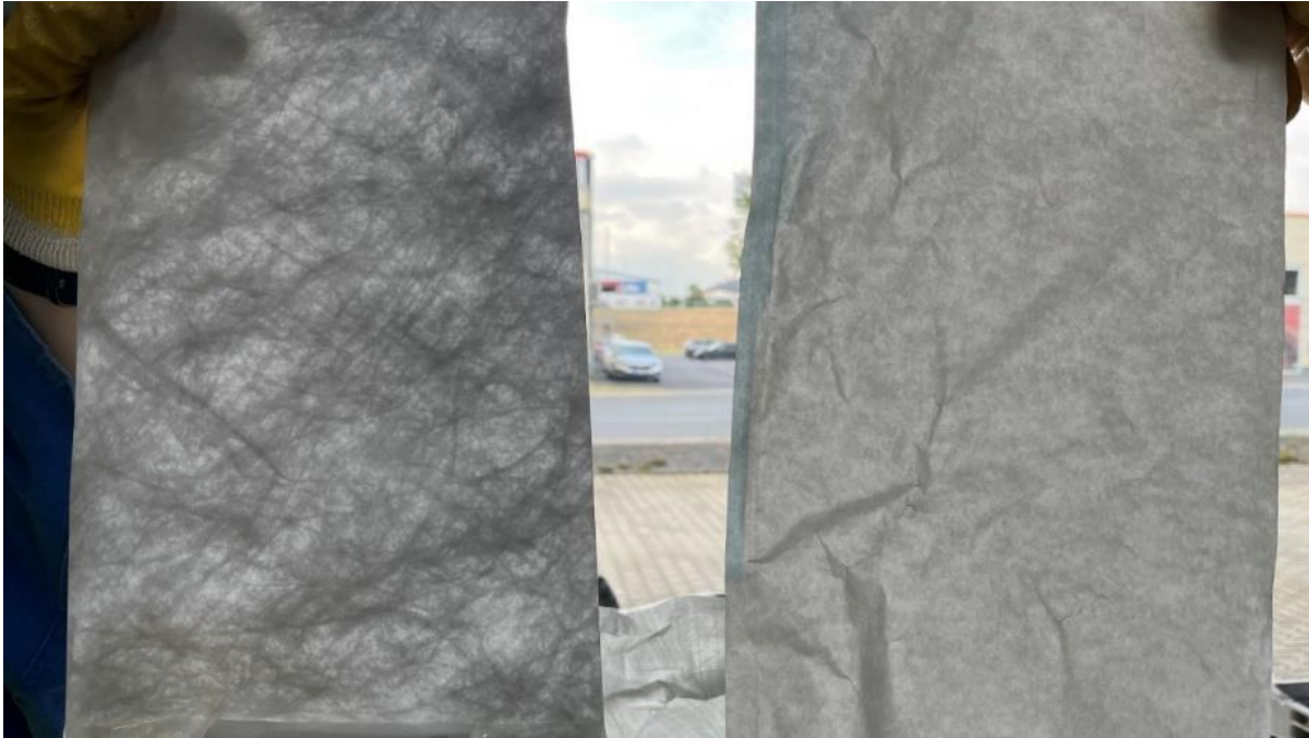
Figure 10. Tyvek® (left) and medical grade paper (right)
