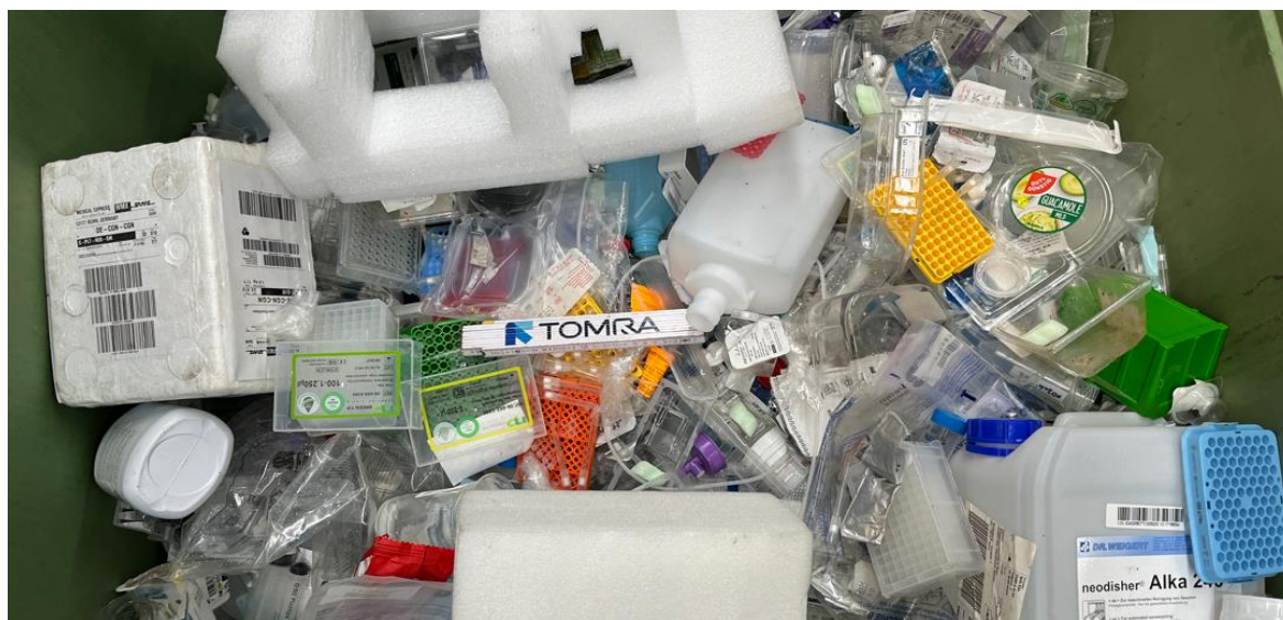
Figure 8. Optically sorted rigid materials output from Step 1 targeting and ejecting PE, PP, and PET
