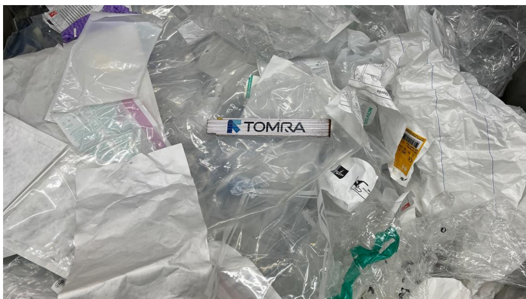
Figure 9. Optical sorting output of PE flexibles
