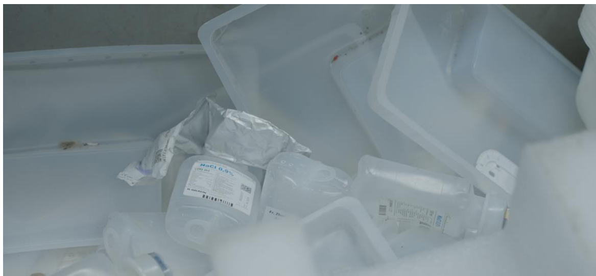
Figure 6. Rigid PP items still containing undersized items like pipets and small test tubes
